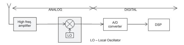
Figure 2. Block Diagram of Software Defined Radio
