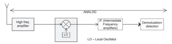
Figure 1. Block Diagram of Analog Receiver
