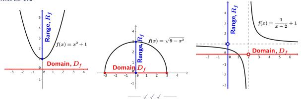
The requirement that a function must assign a *unique* value of the dependent variable to each value in the domain is expressed in the **vertical line test**.
