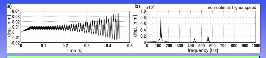
Displacement (a) and its spectrum (b) for non-optimal pair of spindle speed **n=16745 rev/min** and holder stiffness **11000 N/mm**
