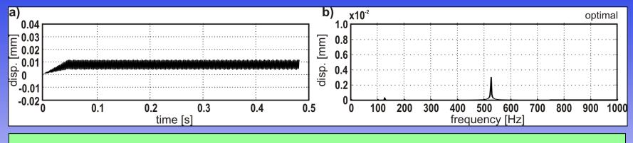
Displacement (a) and its spectrum (b) for optimal pair of spindle speed **n=15745 rev/min** and holder stiffness **11000 N/mm**.
