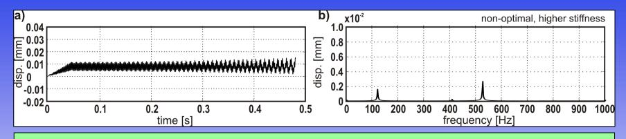
Displacement (a) and its spectrum (b) for non-optimal pair of spindle speed **n=15745 rev/min** and holder stiffness **14800 N/mm**
