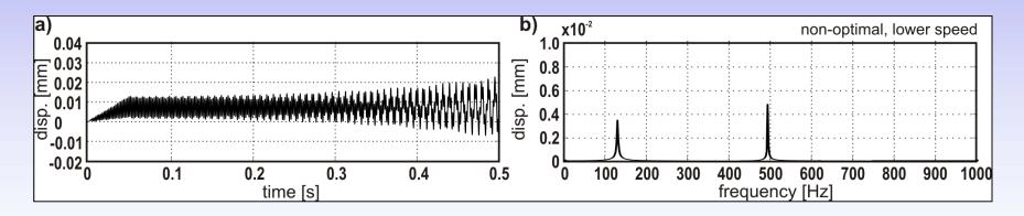
Displacement (a) and its spectrum (b) for non-optimal pair of spindle speed **n=14745 rev/min** and holder stiffness **11000 N/mm**
