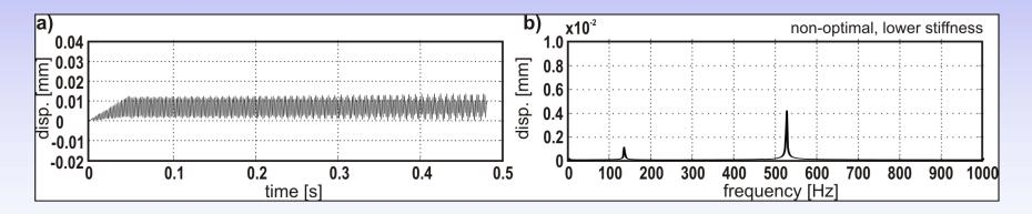
Displacement (a) and its spectrum (b) for non-optimal pair of spindle speed **n=15745 rev/min** and holder stiffness **8500 N/mm**.
